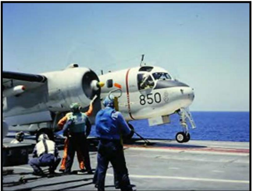
At sea 1972 'UP TOP' (in South East Asia) on patrol during the Cold War. S2E Tracker anti-submarine aircraft 850 from VS 816 Sqn 'Fighting Tigers', set for catapult launch from HMAS Melbourne. Aircraft is armed with 2.75" rocket pods.
